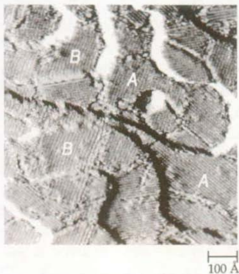
Fig. 3.11 High resolution image of a decanethiol-covered Au(111) surface. Two different types of molecular domains, denoted A and B (see text), coexist on the surface. Tunneling parameters: I = 0.8 \text{ nA} , V = 1.4 \text{ V} .
