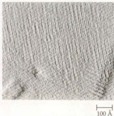
Fig. 3.18 After annealing at 370 K, a transition from the c(4 \times 2) to the striped structure is observed on decanethiol-covered Au(111) surfaces. Tunneling parameters: I = 0.5 nA, V = 0.95 V.
