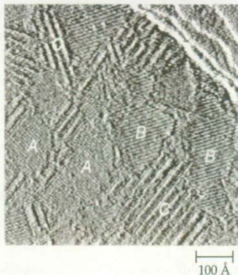
Fig. 3.15 High resolution image of a hexanethiol-covered Au(111) surface. In addition to the A and B structures observed also on decanethiol, a further striped pattern, denoted C, characterizes the surface. Tunneling parameters: I = 1.0 \text{ nA} , V = 1.4 \text{ V} .
