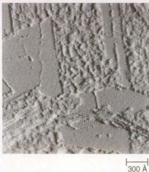
Fig. 4.7 Partially desorbed decanethiol monolayer after 8 hours of annealing at 385 K. Tunneling parameters: I = 0.2 nA, V = 1.0 V.
