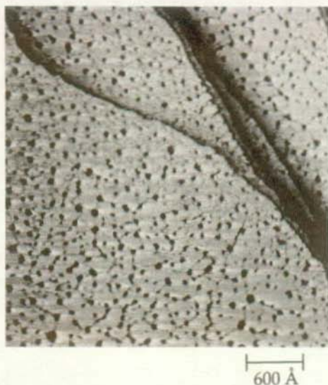
Fig. 3.1 STM image of a decanethiol-covered Au(111) sample at room temperature. A high pit density characterizes the surface. Tunneling parameters: I = 0.5 nA, V = 1.0 V.
