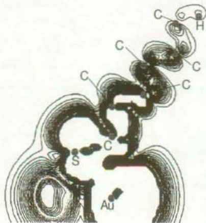
Fig. 3.13 Local electronic density of a hexanethiol molecule on a cluster of three Au atoms integrated in an energy window of 1.5 eV below the Fermi level. Contours from 0.000 to 0.003 electron/(a.u.) 3 (1 a.u. = 0.53 Å) in the plane of symmetry of the molecule (from [Reu]).
