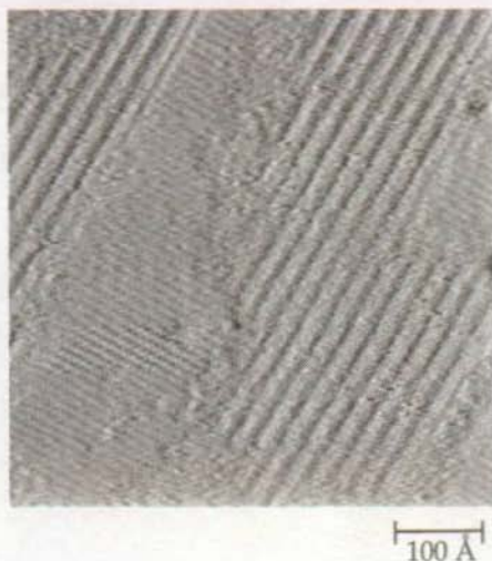
Fig. 3.16 Large uniaxial domains on a hexanethiol-covered Au(111) surface. The percentage of the surface occupied by the striped pattern strongly depends on individual samples. Tunneling parameters: I = 0.3 nA, V = 0.8 V.
