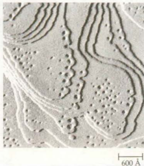
Fig. 3.5 Octadecanethiol-covered Au(111) sample imaged at room temperature after two hours of annealing at 350 K. Pits disappear when they merge with gold steps. Tunneling parameters: I = 0.6 nA, V = 1.1 V.
