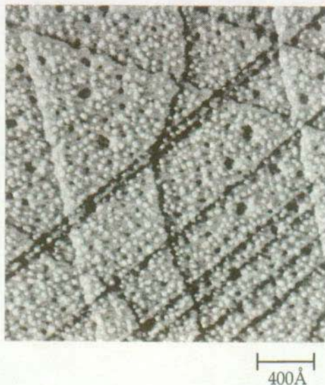
Fig. 5.10 In-situ electrochemical STM image showing the 2D Cu island decoration on a decanethiol-covered Au(111) surface in the UPD potential range. Electrolyte: 50 mM \text{H}_2\text{SO}_4 + 1 mM \text{CuSO}_4 . Electrode potential: 50 mV vs. \text{Cu}/\text{Cu}^{++} . Tunneling parameters: I = 0.3 nA, V = 0.1 V.
