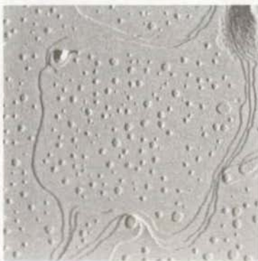
Fig. 4.1 Temporal development of the morphology of a decanethiol-covered Au(111) surface during annealing at 345 K. Tunneling parameters: I = 0.5 nA, V = 1.0 V.
