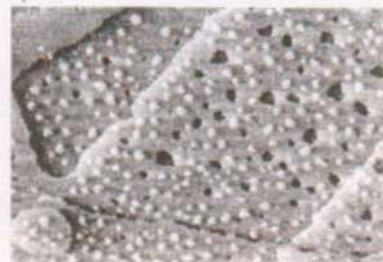
Fig. 5.11 In-situ electrochemical STM image sequence showing the development of the Cu island decoration on a decanethiol-covered Au(111) electrode. Electrolyte: 50 mM \text{H}_2\text{SO}_4 + 1 mM \text{CuSO}_4 . Electrode potential: 150 mV vs. \text{Cu}/\text{Cu}^{++} . Tunneling parameters: I = 0.6 nA, V = 0.05 V.
