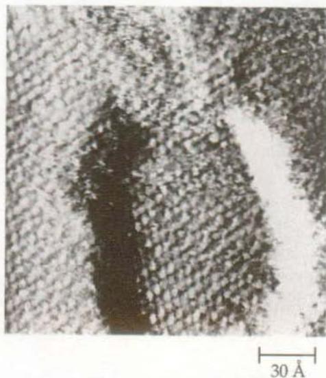
Fig. 3.4 STM image of a decanethiol-covered Au(111) sample. The central part of the imaged region is occupied by a pit. Ordered molecular domains are present inside the hole as well as on the surrounding terrace. Tunneling parameters: I = 0.4 nA, V = 1.1 V.
